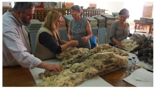
The factory has developed a shoddy-based yarn, with 25% virgin wool. They collect all their waste, on color, and then re-spin this. This yarn will be tested by the Norwegian team.
